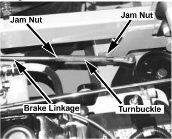
Loosen Brake Linkage Jam Nut Figure 3-10
